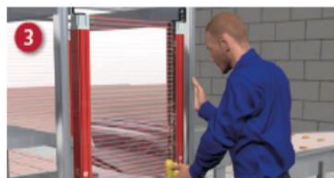
3. Machine operator cleans the light curtain, preventing unnecessary machine downtime.
